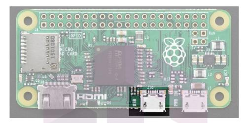
In order to connect a USB device (mouse, keyboard, WiFi) etc you'll need a USB OTG micro B to A cable (http://adafru.it/1099):
